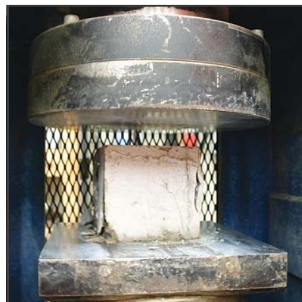
A sample from all batches of concrete produced are bath cured and pressure tested in accordance with ISO 9001
